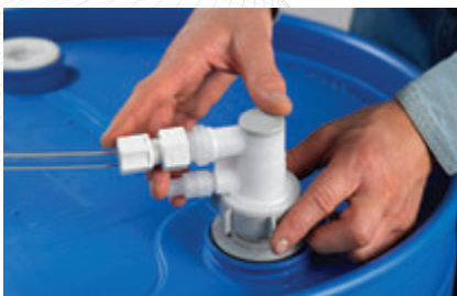
5 Turn the coupler locking ring clockwise until stop is reached (approximately 2 full turns); valve is opened during this process.
