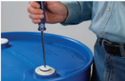
3 Turn shipping plug counterclockwise to remove. (Use a large, flat blade or #4 Phillips screwdriver.)
