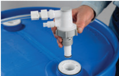
4 Insert coupler into drum insert assembly.
