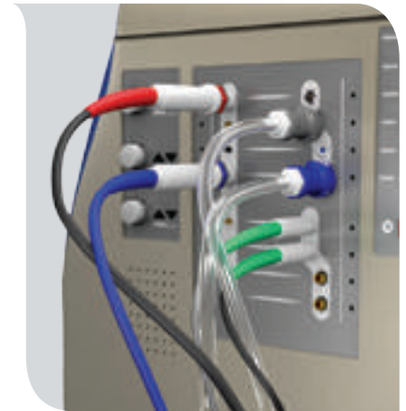
Connections to medical equipment need to be secure and convenient while also preventing misconnections.
