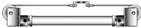
Figure 2 - Cable cylinders can have strokes over 25 feet and can be located remotely from the work load.
