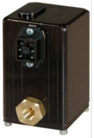
Analog monitor output is standard, select 0-10 VDC or 4-20mA. The dual loop design accepts feedback signal from a wide range of external sensors. The QPV2 accepts feedback signal from F-Series flow transducer for closed loop flow control. It also accepts external feedback of pressure, vacuum or force. Optional digital display is available.
