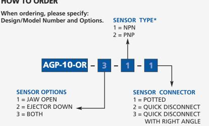
\* NOTE: Proximity sensors are 6.5 mm smooth barrel, 1230 VDC, 50 mA and comes with 2 meter cable.
