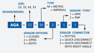
\* NOTE: Hall Effect 4mm dia., 5-24 VDC, 22 mA and comes with 2 meter cable.
