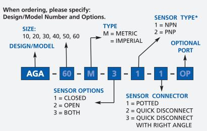
\* NOTE: Hall Effect 4mm dia., 5-24 VDC, 22 mA and comes with 2 meter cable.
