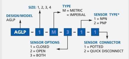
\* NOTE: Hall Effect 4mm dia., 5-24 VDC, 22 mA and comes with 2 meter cable or quick disc.
