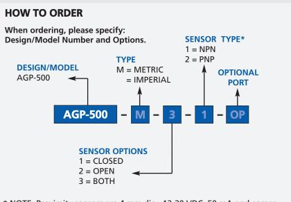
\* NOTE: Proximity sensors are 4 mm dia., 12-30 VDC, 50 mA and comes with 2 meter cable or quick disc.
