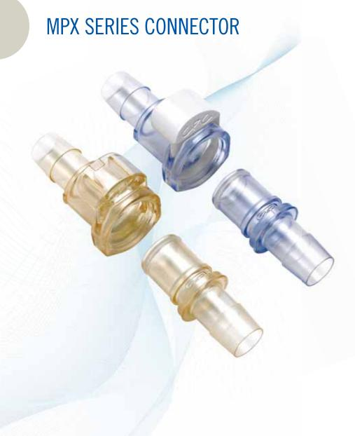
MPX Series couplings add ease of use and security to your most critical fluid handling applications. Choose from a full line of connectors and configurations, including pressure sealing caps and plugs in sizes to fit 3/8" and 1/2" tubing. MPX couplings offer optional locking sleeves to further guard against accidental disconnects. In addition, coupling halves can be rotated when connected reducing tube kinks.
