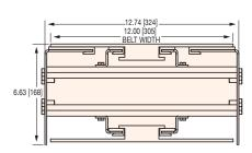
Note: Conveyor modules may be made up of several length of conveyor frames. Maximum length frame is 120" (3048mm).
