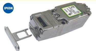
HYGIECAM Series Interlock Switches have a rugged Stainless Steel 316 body and have been designed to cope with the rigorous applications of the Food Processing, Pharmaceutical, Packaging and Petro-Chemical Industries. The surface finish is mirror polished to Ra10 to resist the accumulation of food debris and is suitable for high pressure hosing at high temperature.
