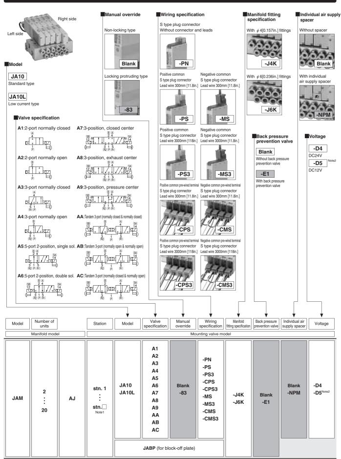
Notes: 1. Valve mounting location is from the left, with the solenoid on top, and the 4(A) and 2(B) ports in front.
