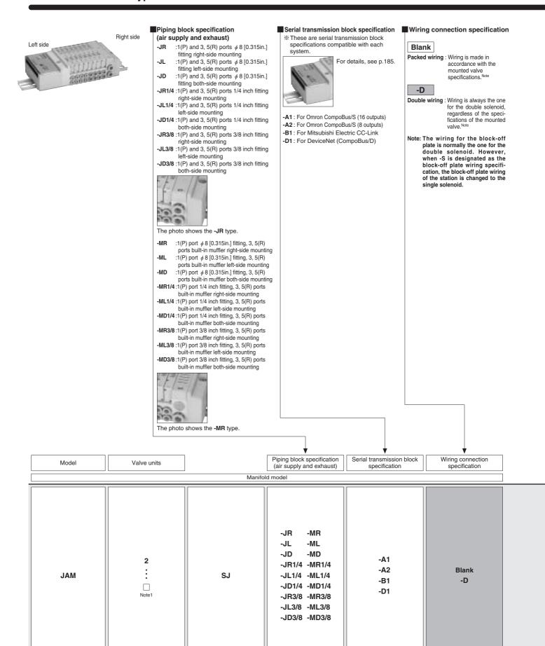
Notes: 1. For the maximum number of units, see the table for the maximum number of valve units by serial transmission block specification, on p.203.
