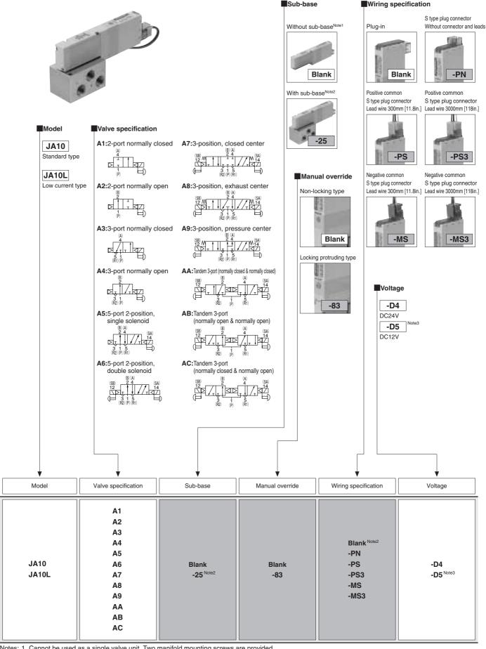
Notes: 1. Cannot be used as a single valve unit. Two manifold mounting screws are provided.
