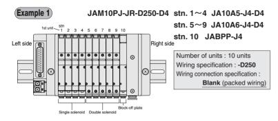
Caution: For the sake of convenience, the connector pins are assigned based on the solenoid valve wiring sequence. which differs from the pin locations and pin numbers (marked) prescribed in JIS-X5101 for the data circuitterminating equipment (DCE).
