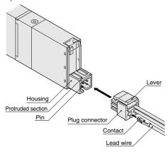
Caution: When removing the connector, confirm that the lever claw is completely disengaged from the protruded section before pulling out. The housing may be damaged if it is pulled out while engaging with the protruded section
