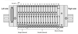
Caution: For the sake of convenience, the connector pins are assigned based on the solenoid valve wiring sequence, which differs from the pin locations and pin numbers (marked) prescribed in JIS-X5103 for the data circuit-terminating equipment (DCE).
