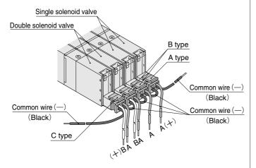
For common connector assembly, order the common connector assemblies listed below.
