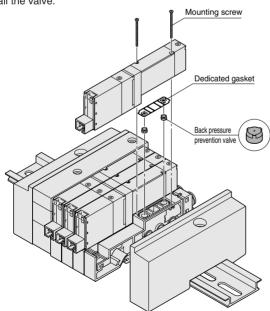
Tightening torque of mounting screw : 17.6N⋅cm {1.8kgf⋅cm} [1.56in⋅lbf]
