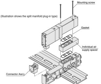
Remark: When attaching fittings to the Individual air supply spacer, use the recommended fittings shown below.
