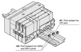
Caution: Mounting port isolators requires disassembly and re-assembly of manifolds.
