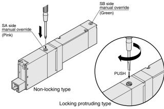
Cautions: 1. The JA series valves are pilot type solenoid valves. As a result, the manual override cannot switch the main valve without air supplied from the 1(P) port.
