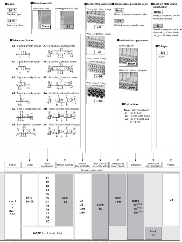
Notes: 2. Valve mounting location is from the left, with the solenoid on top, and the 4(A) and 2(B) ports in front.
