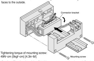
Caution: The direction of the -D370U connector cannot be changed, D-sub on top is the only option.
