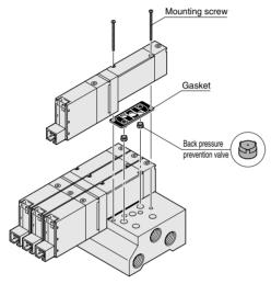
For the split type manifold, remove the gasket from between the valve and manifold, insert the back pressure prevention valve into the exhaust port, mount the dedicated gasket provided, and then install the valve.
