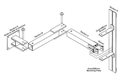
Excellent method of mounting light curtain on press brakes or when light curtain is to be removed for die setups or machine maintenance. Model 9000 consists of three 180 degree pivot points along with light guard diagonal movement capability for virtually unlimited light guard positioning. Two-inch square tubing (3/16" or 4.76mm thick) painted OSHA yellow which mounts directly onto the machine housing and makes for a heavy duty, yet versatile mounting bracket. Specify dimensions "B" and "C."
