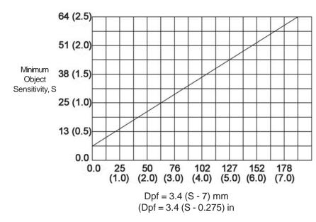
Penetration factor, Dpf, for presence-sensing devices used in a vertical application with object sensitivity less than 64 mm (2.5 inches)
