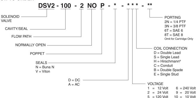
Omit coil for cartridge only with nut.
