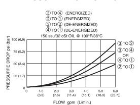
**Operating Pressure:** 3000 PSI (207 Bar) **Flow:** See PRESSURE DROP VS. FLOW graph.
