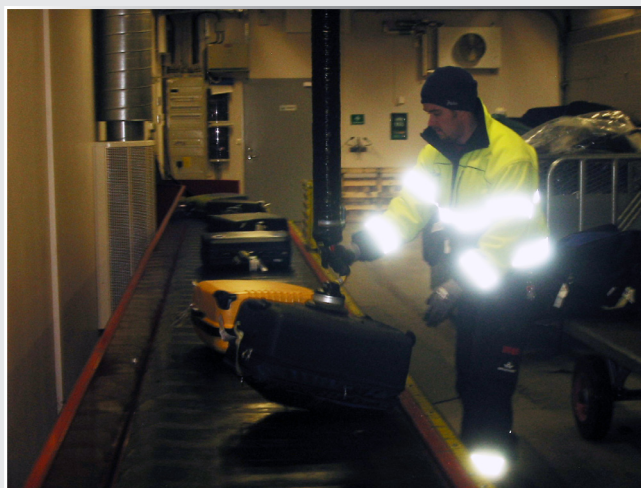
Vacuum lifters can be used to eliminate manual handling in the airport baggage handling areas. VacuCobra lifts baggage of different size and shape weighing up to 50 kg.
