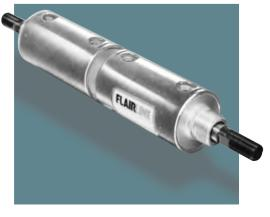
Cap-to-Cap models consist of two F, O, H or D type cylinders joined at the cap end by a common center section. Each unit can be operated independently of the other to accurately attain and repeat three positions when both units are the same stroke and four positions when each unit is a different stroke. See page 7 for dimensional data and page 10 for mounting accessories. For special options, see page 16.
